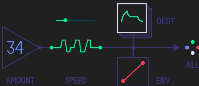
Blue encoder sets Amount. Green encoder sets speed. White sets Destination and Orange encoder sets the envelope Attack / Decay.
