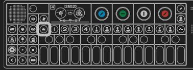
To add a master effect, press the T3 key. You may toggle an effect on and off by pressing the T3 key a second time.
