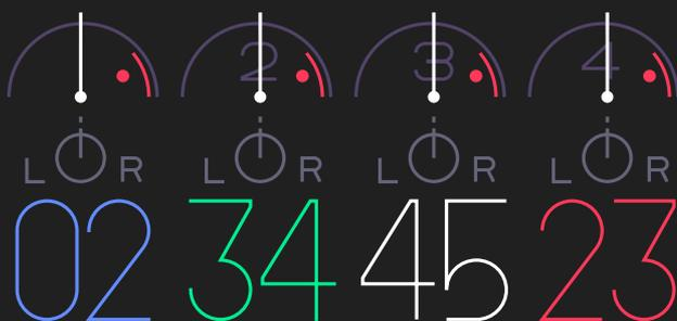
In the Mixer main screen, you adjust the individual level and Pan Left / Right of Tape tracks 1-4
