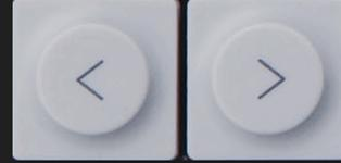
In tape mode:   Bar step back   Bar step Forward
