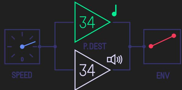
Blue encoder sets Speed. Green encoder sets Pitch. White encoder sets Volume and Orange encoder sets the envelope Attack / Decay.
