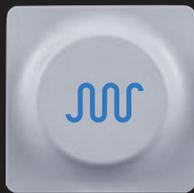
To enter Synthesizer Mode, press the key with the blue wave symbol on it. This enables both T1-T4 and sound selection keys 1-8. When you have pressed the Synthesizer key, first select a sound from 1-8 with the Sound keys:
