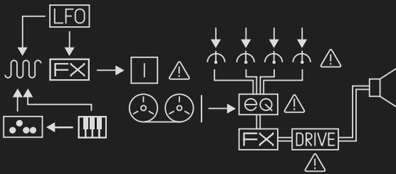
NOTE: A warning symbol will lit up when any critical level is set to zero.
