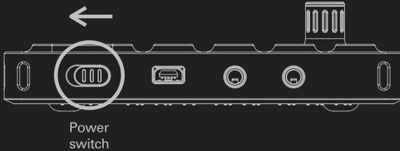
To power off, slide the power switch upwards. Data is always stored on-the-fly, so you don't have to worry about saving your sound or recordings.
