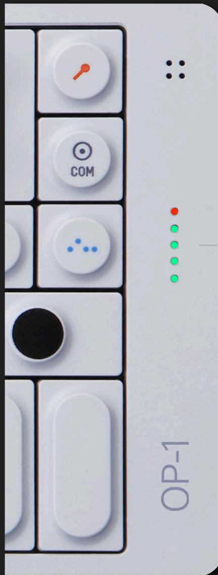
The Battery level is indicated by the LED array on the right side of your OP-1. All LED's lit (including the red) indicates a fully charged battery good for around 16 hours of heavy use. The stand-by time is approx. 2 years.
