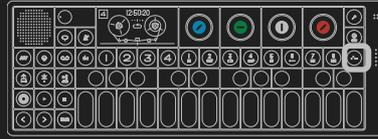
**NOTE:** To key transpose a Pattern sequence, switch to Synthesizer, Drum, Tape or Mixer mode and press any key on the Musical Keyboard. To play the original pitch of the sequenced notes, play the C key on the Musical Keyboard.
